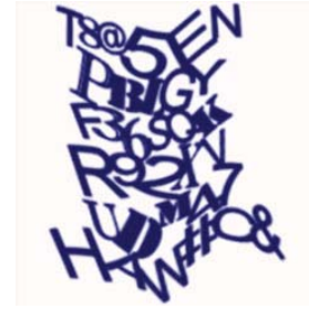
Figure 5. Screenshot of the graphical password keyboard. The user clicks his password and the click positions are used to check if the password is correct. This alone can be seen as a prevention based mechanism. For a classical click-based CAPTCHA, apart from the “keyboard” also the “password” would be provided (source: [22]).
