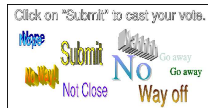
Figure 6. A screenshot of an implicit CAPTCHA that allows to solve it with a single click. The goal is to click on the word Submit (source: [23]).
